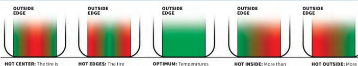
HOT CENTER: The tire is likely overinflated, raising the center and reducing friction and traction on the outside and inside. This can lead to overheating the rubber and excessive sliding.
