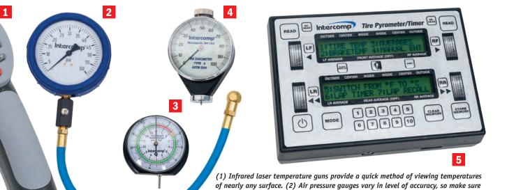
to use a high-quality gauge for your data collections. (3) Tire tread depth gauges help to monitor the lifespan of your tires in fine detail. (4) Tire durometers measure the softness of a tire, which can change in relation to temperature. (5) Digital gauges allow you to quickly measure and store information in an organized manner.
