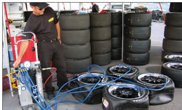
Intercomp’s Tire Drying/Purging System allows racers the ability to simultaneously remove water vapor-contaminated air from a set of tires, and replace it with pure nitrogen.
