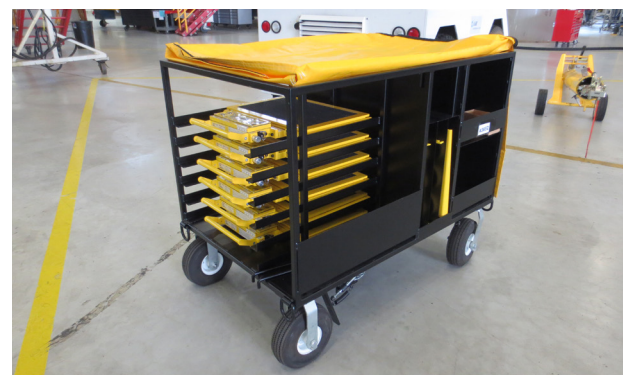
The compact cart requires minimal space, and stores the full weighing kit in a self-contained, easily towable cart.
