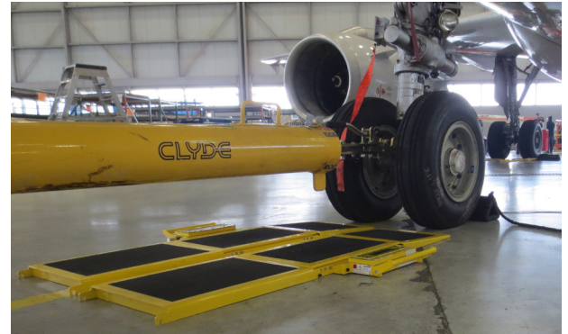
Low-profile scales minimize towing distance, with overrun spacers further increasing safety during weighing.
