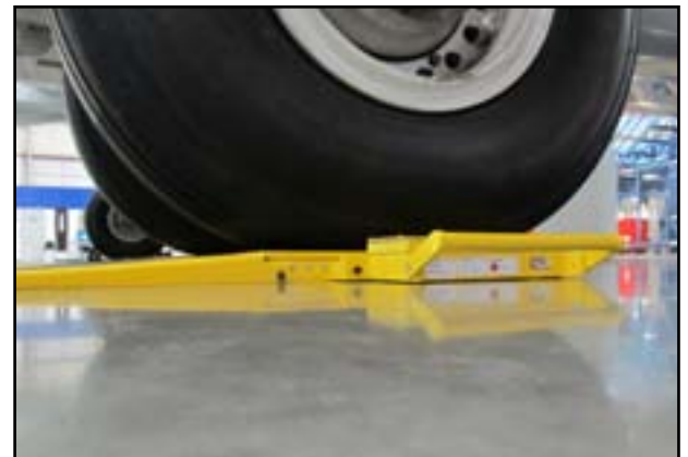
Low-profile scales enable short towing distances
