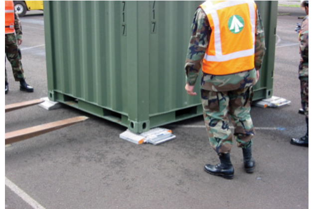
Utilizing portable PT300™ Wheel Load Scales in each corner of a container is an economical way to verify fully loaded containers. (SOLAS Method 1)
