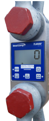
Tension links with simple wireless operation and easy-to-read display.
