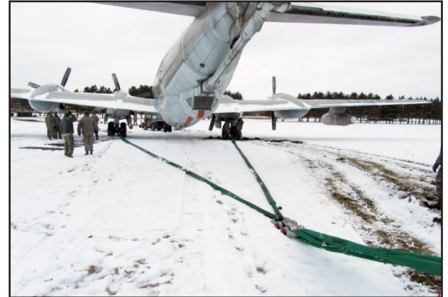
Typical use: Load monitoring on towing straps connected to landing gear.
