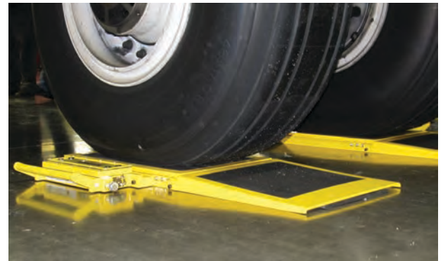
Low-profile scales are certified intrinsically safe for use in hangars.
