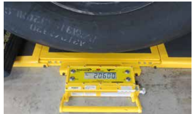
The fully-electronic, intrinsically safe scales provide stable, repeatable readings on an easy-to-view screen.
