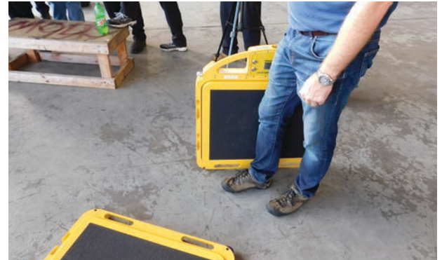
Single-person portability with integrated wheels enable rapid deployment of scales.
