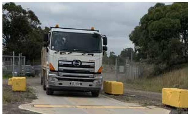
LS-WIM ® Scale systems provides an efficient method to weigh trucks in high-traffic locations.
