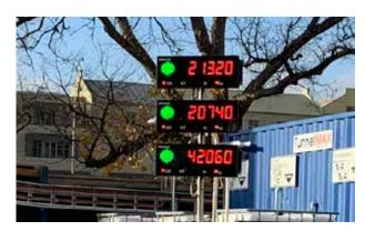
LED displays allow the driver to view live axle weights to keep from leaving the worksite overloaded, or causing inefficiencies due to an under-loaded truck.
