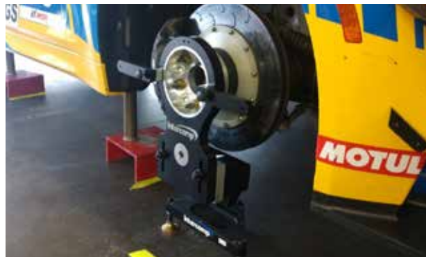
By utilizing custom machined hub adapters, Intercomp's HUBSCALE360™ features a solid, precise fit for racecars with a variety of designs including production-based 5-lug hubs.
