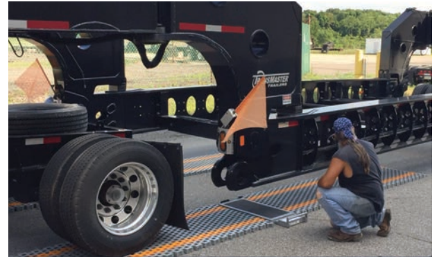
The LS630-WIM™ System is the most efficient means to weigh multi-axle truck/trailer combinations, recording up to 36 individual axle weights per vehicle.
