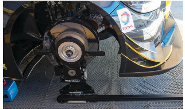
Intercomp's Precision Hub Scale System further removes variables, such as setup tires, from the process of measuring corner weights of high-end racecars.
