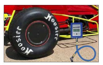
An Intercomp Digital Air Gauge provides the ability to set to the optimal tire pressure and fine-tune a racecar's handling.
