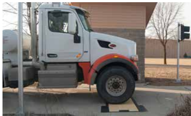
The LS-WIM System can be operated without the need for a gate operator. The driver is responsible for entering a code, or using a key fob to activate the system.
