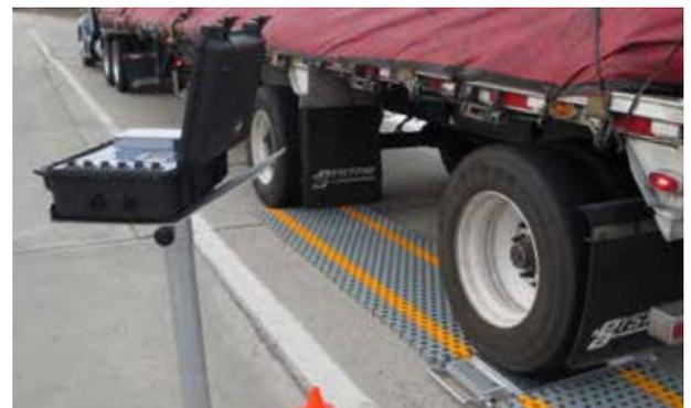
The LS630-WIM™ scale pads can connect to an indicator using either cables or RFX™ Wireless Weighing technology, creating the ideal scale system for nearly any jobsite.
