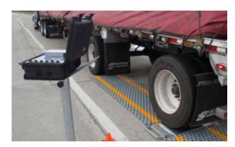
The LS630-WIM™ scale pads can connect to an indicator using either cables or RFX™ Wireless Weighing technology, creating the ideal scale system for nearly any jobsite.
