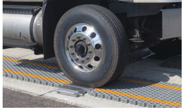
The scales can accommodate a variety of single-lane width vehicles, up to 36 axles.
