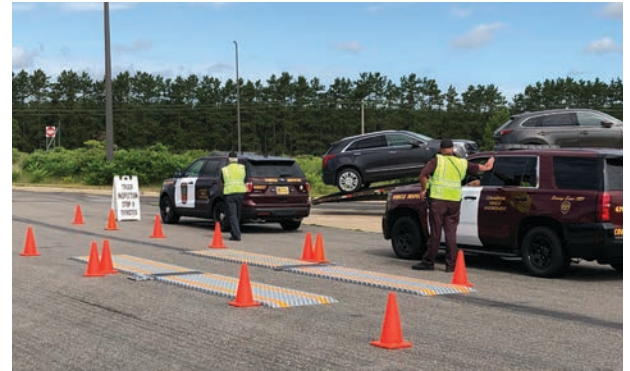
Portable WIM system is deployed where vehicles enter the temporary enforcement site.
