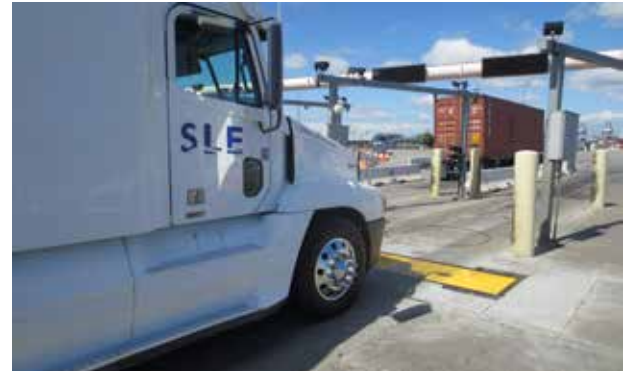
Intercomp LS-WIM in-ground axle scales minimize backups at the Port of Los Angeles by allowing incoming and outgoing traffic to continue moving.
