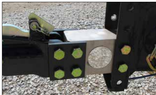
Subsequent updates included a ladder hitch load cell replacing the original round bar, making it simpler to adjust the height, and decreasing install time even further.
