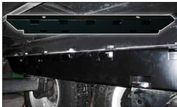
The Intercomp Beam Scale is a drop-in replacement for the original (non-scale) channel in the seed tender's frame and uses the same bolts and mounting hardware as the standard channels.
