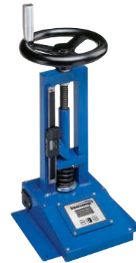
The crank-style Valve Spring Tester allows the user to compress a spring to a particular height, then record the force value without losing pressure on the spring.
