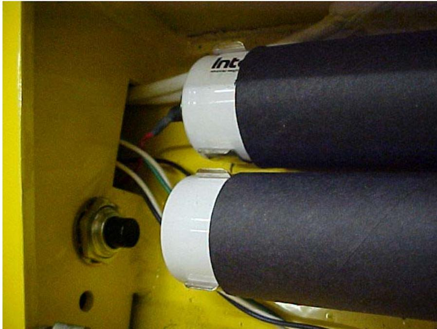
**Figure 2** AC30 battery compartment, showing the setup button
