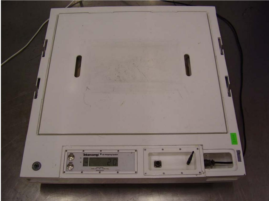
**Figure 3** AC30 with mains power supply and RF transceiver
