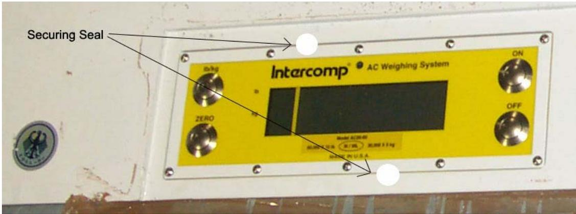
**Figure 6**      **Alternative sealing arrangement**
