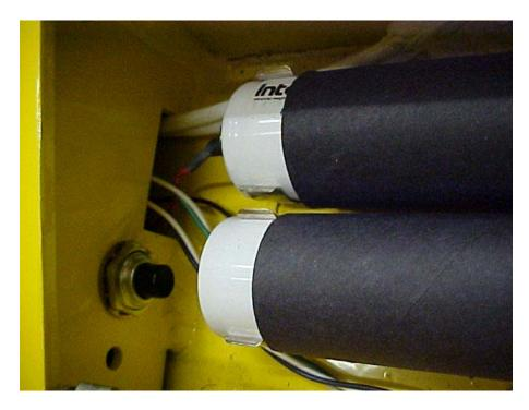
Figure 2 AC30 battery compartment, showing the setup button
