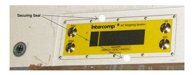
Figure 6 Alternative sealing arrangement
