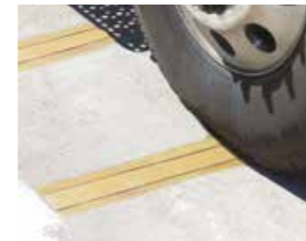
(Left) Portable LS630 WIM scale (Above) Intercomp's WIM strip sensor
