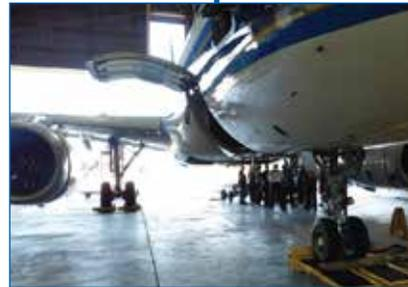
What are we actually doing when we weigh an aircraft? What does it all mean? When we weigh an aircraft, for whatever reason, we are looking to update its basic weight and associated center of gravity. The importance of Operating Empty Weight (OEW), Manufacturer's Empty Weight (MEW), and weight of Standard and Operator Items (SI & OI respectively) are clear with the following equation:
