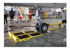
your scales, which is much safer than pushing the aircraft. Once the scales are exercised to the full weight of the aircraft, zero your scales prior to your first actual weigh. If you feel you need to chock your aircraft once up on
