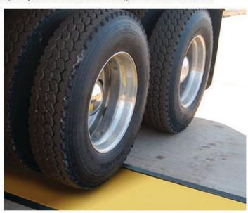
The 13-square foot area of the LS-WIM weighbridge equates to a smaller installation and operation footprint than required by full-length truck scales.
