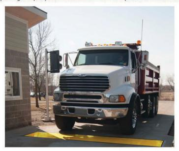
A 13-foot wide weighbridge minimizes importance of wheel placement for accurate weighing and allows for measurement of virtually any single lane-width vehicle.
