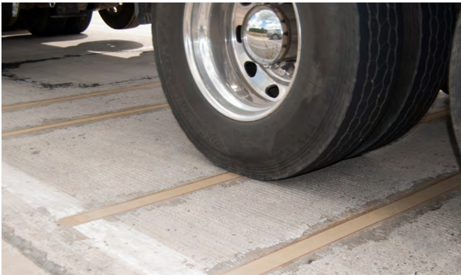
Strip Sensors bundle low installation and maintenance costs, with the ability to weigh moving vehicles at any speed, into a flexible and dependable package.
