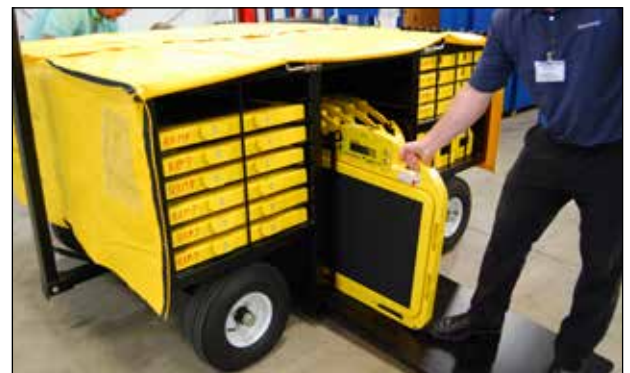
The AC60-LP™ comes in a kit with spacers for different types of aircraft, and is rapidly deployed without ever lifting a scale.
