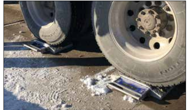
Using two scale pads under all wheels in an axle group allows the weight to be distributed evenly between the two axles.
