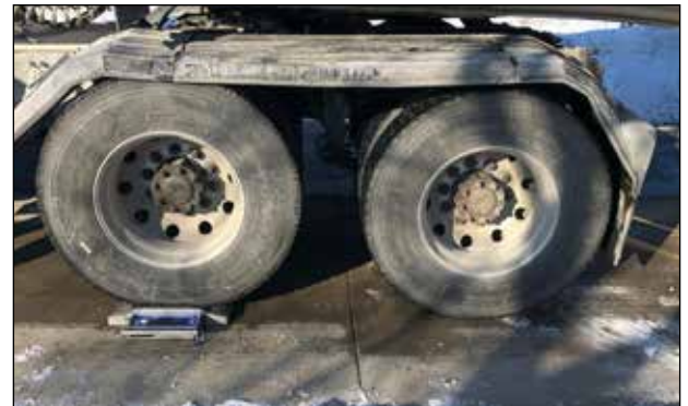
By using a pair of scale pads on one axle in a group, the compressed suspension shifts weight toward other axles in the group.
