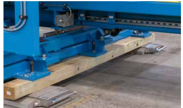
RFX® Wireless Weighing Technology allows a scale operator to read the total weight recorded by all four pads at the push of a button.
