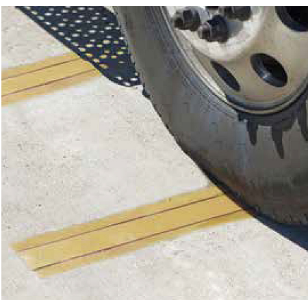
Strain Gauge-based Strip Sensors offer improved accuracies for Gross Vehicle Weights and Axle Weights versus piezoelectric sensors.
