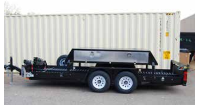
The AX900™ Axle Scale Trailer is a reliable and durable option for transporting AX900™ scales to areas not served by permanent truck scales.
