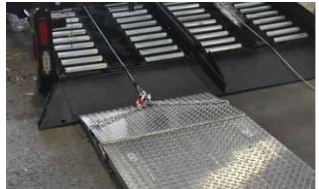
The trailer is equipped with scale rollers, winches and a hydraulic tilt package which virtually eliminate the need for manual labor when pulling the scale up the trailer.
