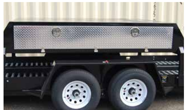
Toolboxes and overhead storage provide additional space for associated equipment, signage, and other needs of the enforcement officers.
