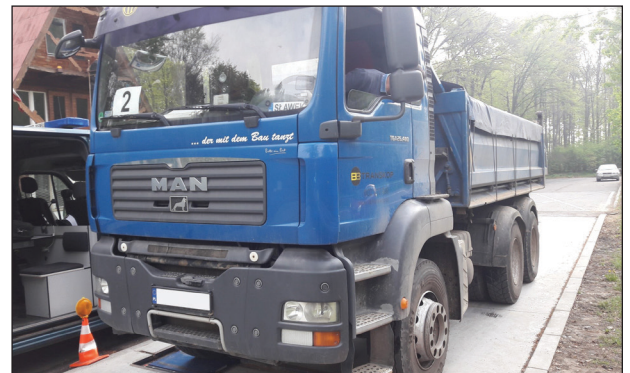
The 3-axle, 24T vehicle tested with a single axle and 2 axles in a group.
