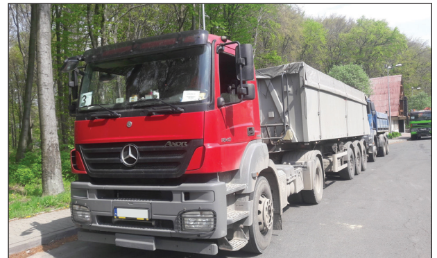
The 5-axle vehicle with trailer, consisting of 2 single axles and a 3-axle group.
