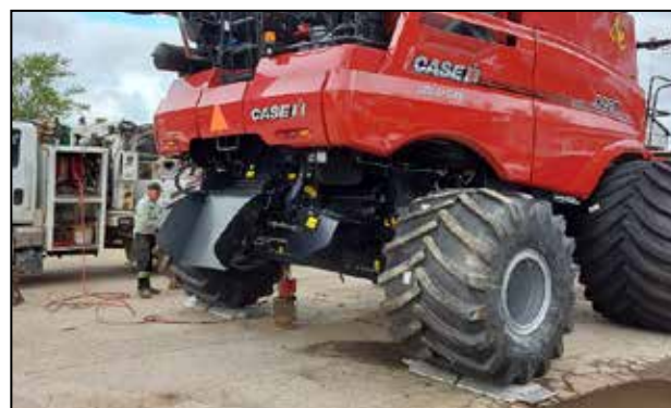
Built-in wireless technology allows the viewing of weights from a safe location rather than crawling underneath large equipment to read the scale indicator.
