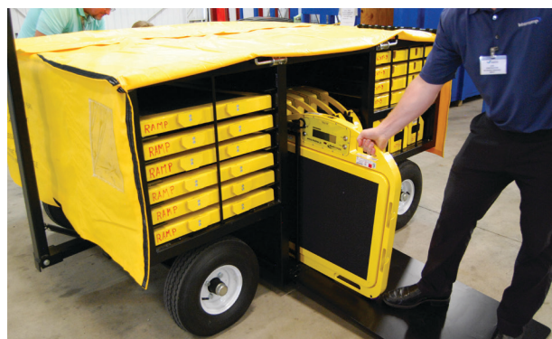
Carts transport and store the kit with integrated ramps, so there is no need to lift scales.
