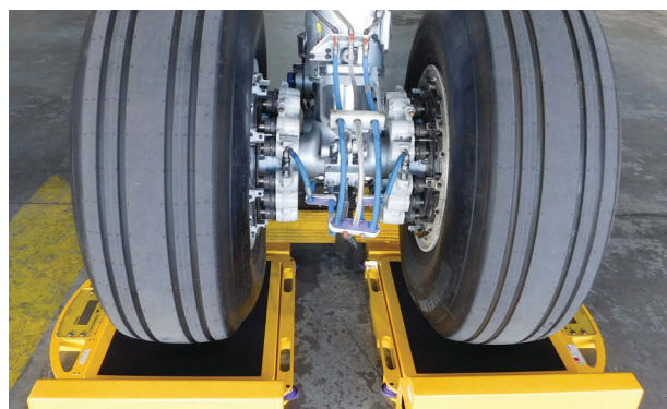
AC60-LP™ low-profile intrinsically safe aircraft platform scales.
