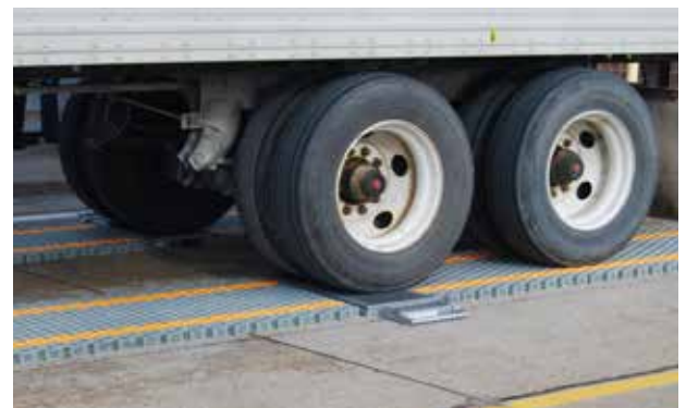
Ramps keep axle groups on level, with large scale surfaces allowing for weighing dual tires easily.
