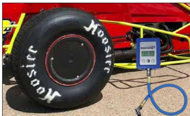
An Intercomp Digital Air Gauge provides the ability to set to the optimal tire pressure and fine-tune a racecar’s handling.
