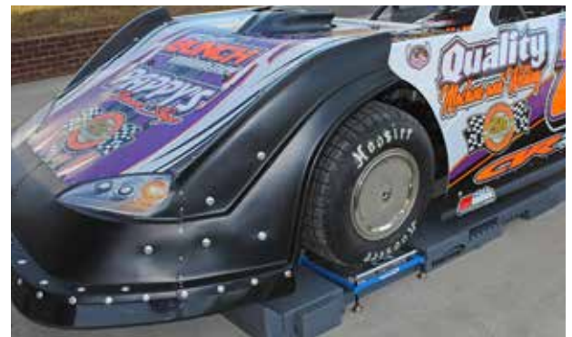
A Late Model racecar is corner balanced on a set of RFX™ Wireless scale pads and Quik Ramp lightweight, modular scale rack.
