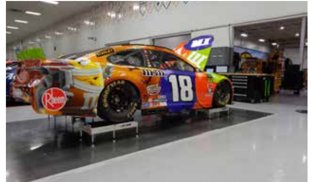
The Joe Gibbs Racing No. 18 NASCAR Cup Car is weighed on Intercomp Microflex™ RFX™ Wireless scale pads set in Billet Levelers with Roll-Off Pad in the team’s Huntersville, NC shop.
