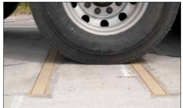
WIM Strip Sensors are installed into channels cut into the pavement, and are used at speeds ranging from 3-120+ km/h.
