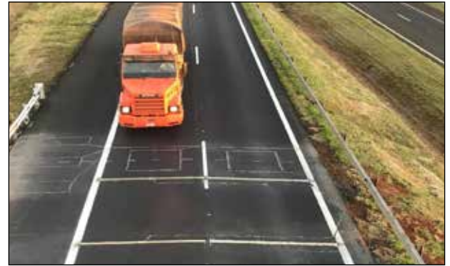
Two pairs of Intercomp Strip Sensors are installed to cover the width of each lane to provide the desired accuracy.
