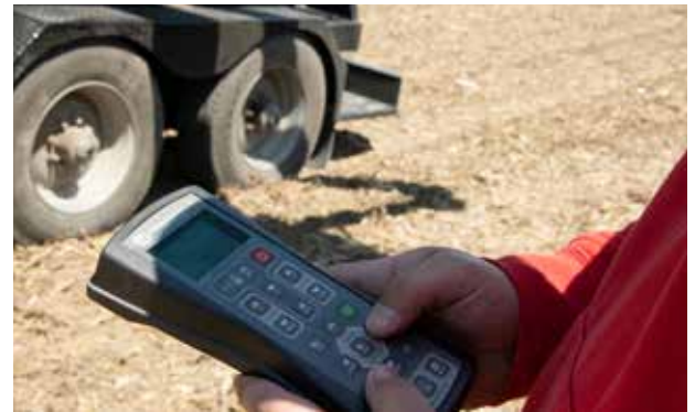
The HH520™ RFX® Wireless Handheld device can control up to 26 equipment functions and allows an operator to control the system from the most convenient location.
