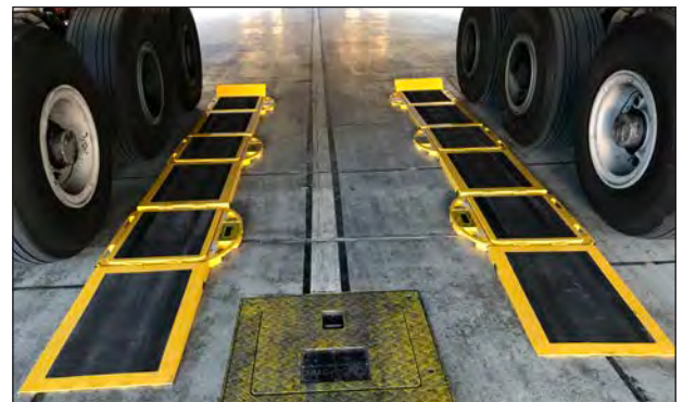
Wireless, low-profile AC60-LP™ scales for the A380 main landing gear
