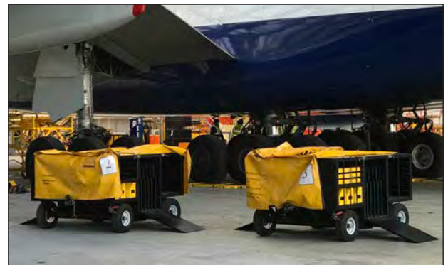
Carts store ramps, spacers, stops, and platform scales with integrated wheels, with ramps for rapid deployment
