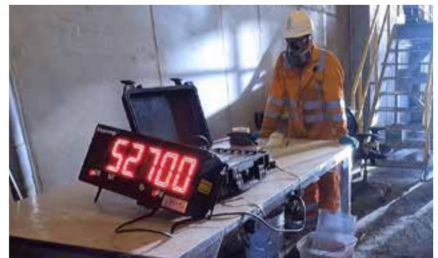
Intercomp's LED Remote Display shows the accumulated weight as copper concentrate as the truck is loaded.
