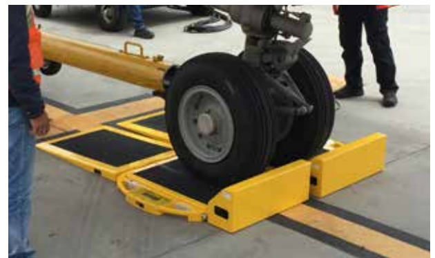
Low-Profile AC60-LP™ scales have large active weighing platform to weigh many aircraft types.
