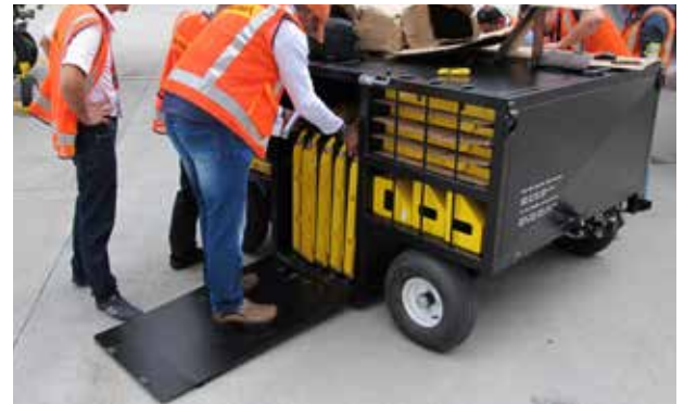
Rapidly deploy aircraft scales from transport cart with ramps, without needed to lift scales.
