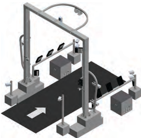
Automated gate kiosks and optical recognition technologies improve not only the efficiency of terminal movement, but also the accuracy and security of operations.
