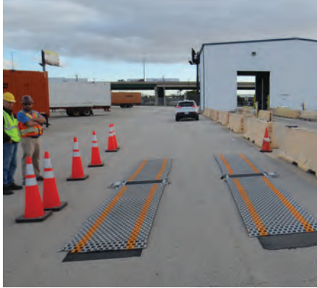
The rail carrier used Intercomp's LS630-WIM™ portable scale to evaluate the benefits of integrating Weigh-In-Motion technology into their new automated gates.
