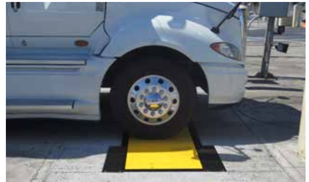
The low-speed Weigh-In-Motion system weighs each axle as vehicles drive over a weighbridge at speeds of 5-10 mph.
