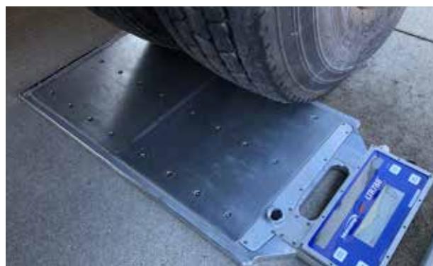
The LTR788™ Dual Wheel Load Scale has a split weighing platform for direct measurement of individual tire loading within dual-tire configurations.
