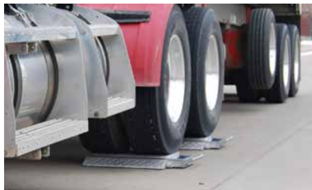
Individual tires in dual-wheel configurations were assumed to carry near equivalent loads because the default procedure for measurement was weighing both tires together and dividing by two.
